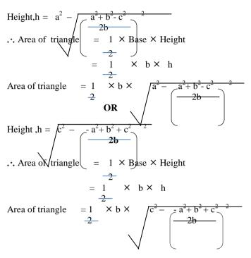
From above two new formulae, we can find out the height & area of any types of triangles.
